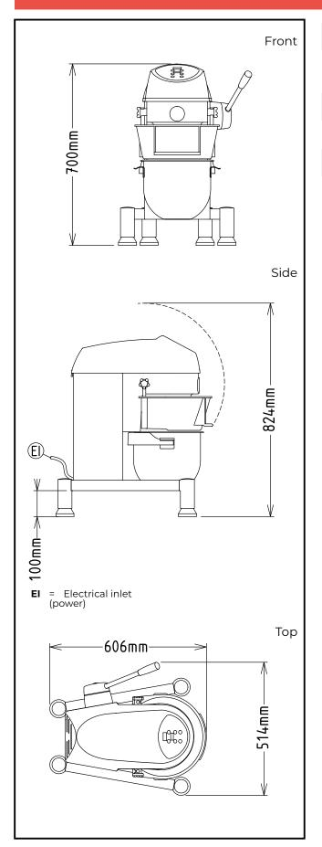
Electric Supply voltage: 380-415 V/3 ph/50 Hz Electrical power, max: 0.5 kW **Total Watts:** 0.5 kW Capacity: Performance (up to): 3.5 kg/Cycle Capacity: 10 litres Key Information: External dimensions, Width: 454 mm External dimensions, 606 mm Depth: External dimensions, Height: 700 mm **Shipping weight:** 57 kg Net weight (kg): 45 **Cold water paste:** 3.5 kg with Spiral hook
